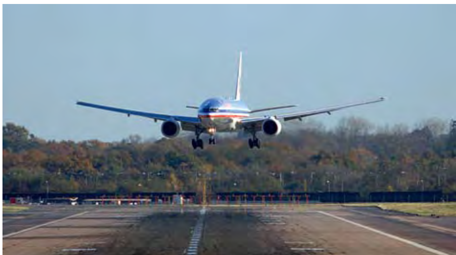
Even airliners have to consider the crosswind and be able to correct the crab angle for landing.
