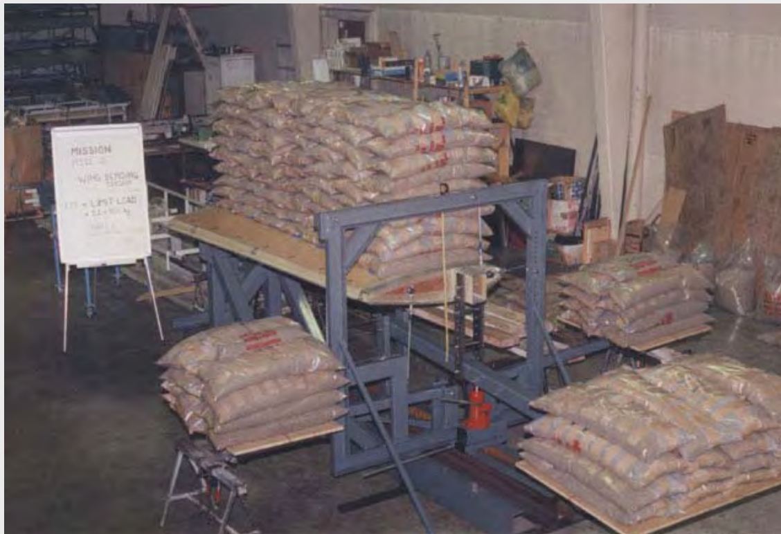
Structural Testing Program: wing test to ultimate load
