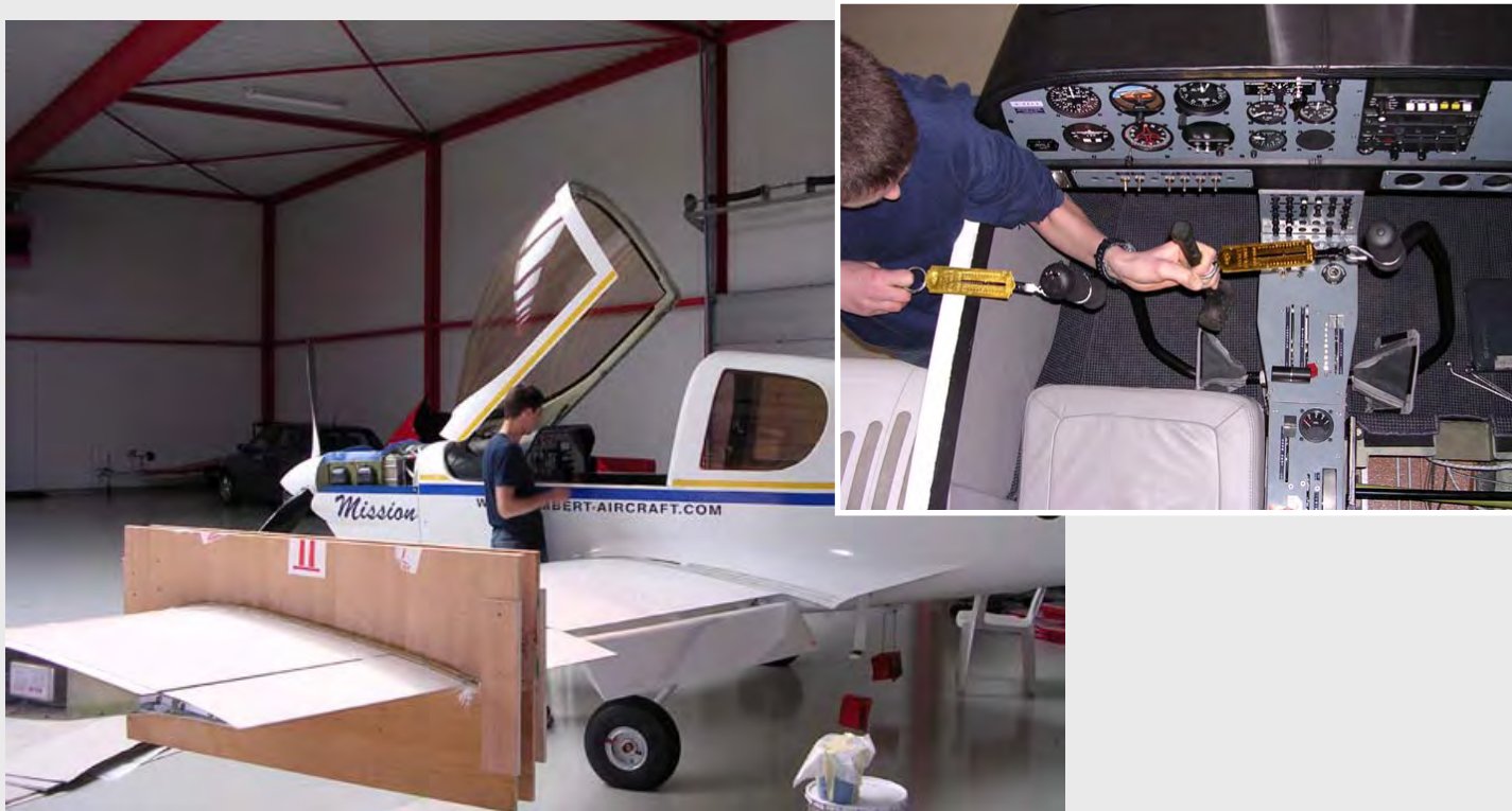
Structural Testing Program: control system test
