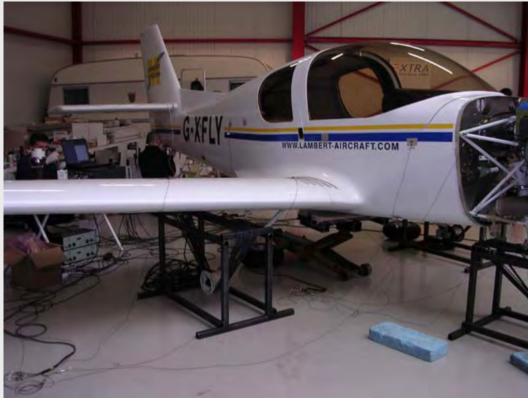
Ground vibration tests being prepared
