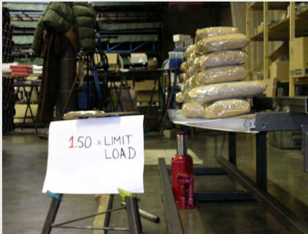
Structural Testing Program: control surface test
