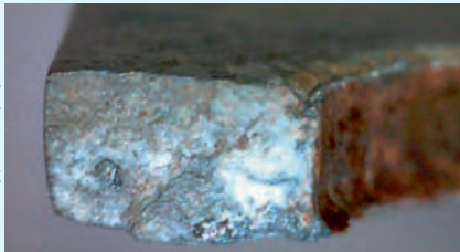
Fracture face of the MCR-01 flap bracket. Note corrosion (white stuff), fatigue beach marks (left lower corner), and the typical 'cup and cone' (cone showing, lower centre).
