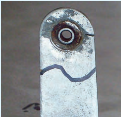
Failed flap bracket – crack at three o'clock.
