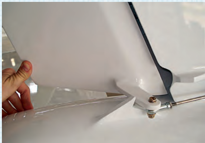
Here's one that is likely to jam; note the overlap. The LAA will shortly be issuing an updated AIL offering advice to owners of Jabiru aircraft about this matter, but it is essential that pilots of all aircraft ensure that the control surfaces are free to move and that there is no possibility of a jam.
