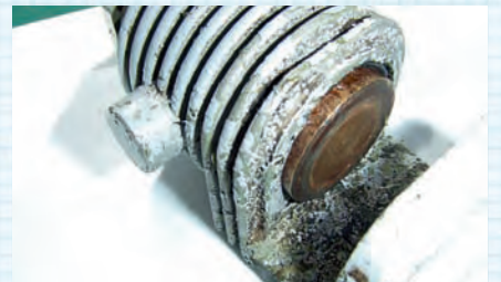
You can see Cedric's problem: the inner edge of the brake calliper has disintegrated, exposing the 'O' ring surface. This brake unit is only four years old, and may have been missed without complete disassembly. It is essential that calendar life of components is taken into account in your maintenance schedule.
