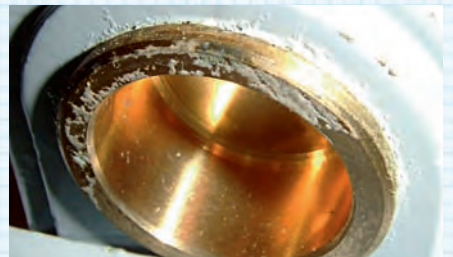
This is worrying. There were signs of corrosion on this replacement part before it had even been fitted. Several Eurostars operate under an LAA Permit; this is the first time I've seen this.
