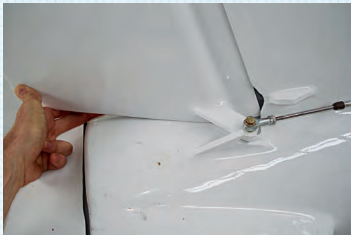
This is a photographic example that shows an acceptable rudder fit. No matter how much the fin/rudder assembly may move about, there is absolutely no way that the leading edge of the rudder can foul against the trailing edge of the fin.
