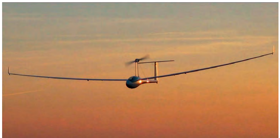
Antares' propeller turns at a maximum of 1700rpm, with implications for both noise and efficiency.
