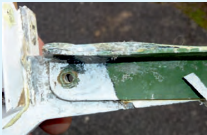
Notice the distinct line between corroded and non-corroded metal, due to weather exposure.
