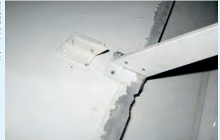
Water played a primary role in this corroded trailing edge, as the joint was covered by tape.
