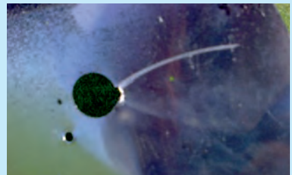
Tell-tale scratch (and dent) left by the throttle cable attachment on an Ikarus C42 aircraft. The throttle is a primary aircraft control and a throttle jam could cause a serious accident.
