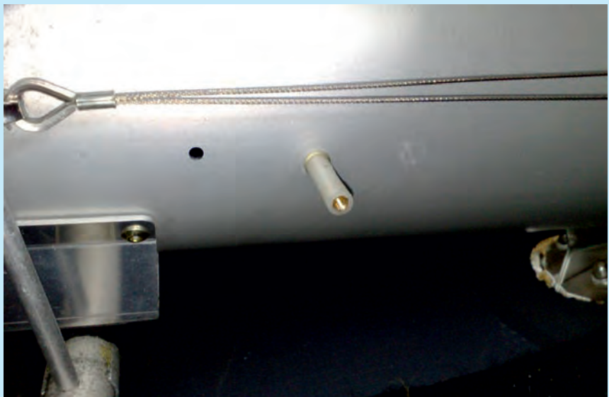
A simple mod devised to keep the side panel away from the throttle mechanism.
