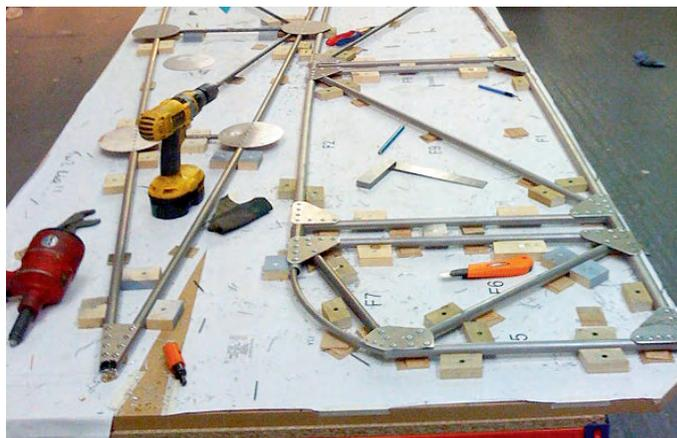
The fuselage components are laid out on full-sized plans and riveted together with pulled rivets using basic hand tools.
