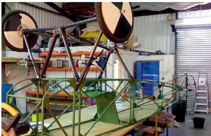
The inverted fuselage with assembled chromolly tube landing gear complete with large-diameter spoked vintage-style wheels.
