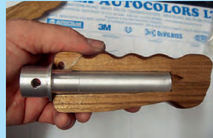
This is the mod incorporated to spread the load a little better into the control stick.
