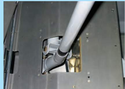
The fact that the second stick on this RV9A wasn't secured with a bolt may have seemed like a good idea at the time; easy to remove, to make space for baggage for example. Trouble was, it fell out during the landing flare while being flown from the P2 seat.
