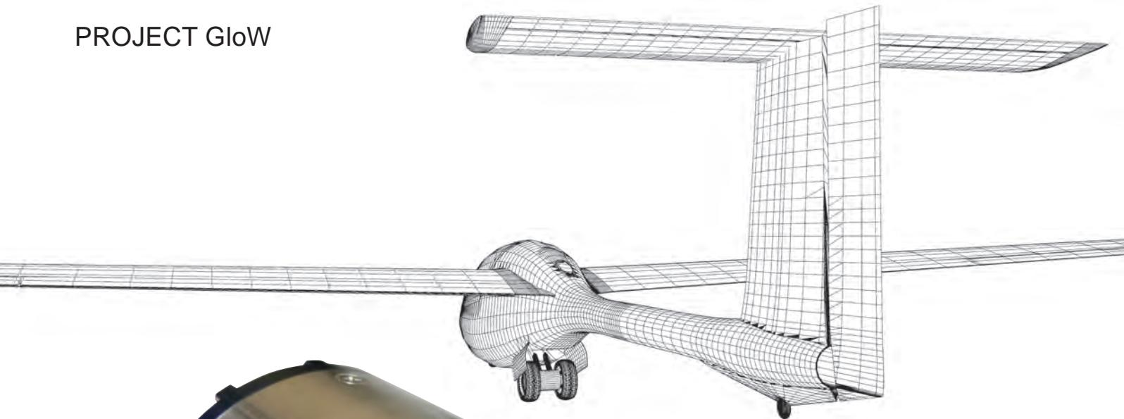
An earlier 'wire' computer image shows the outlet for the jet thrust and the driven wheel arrangement
