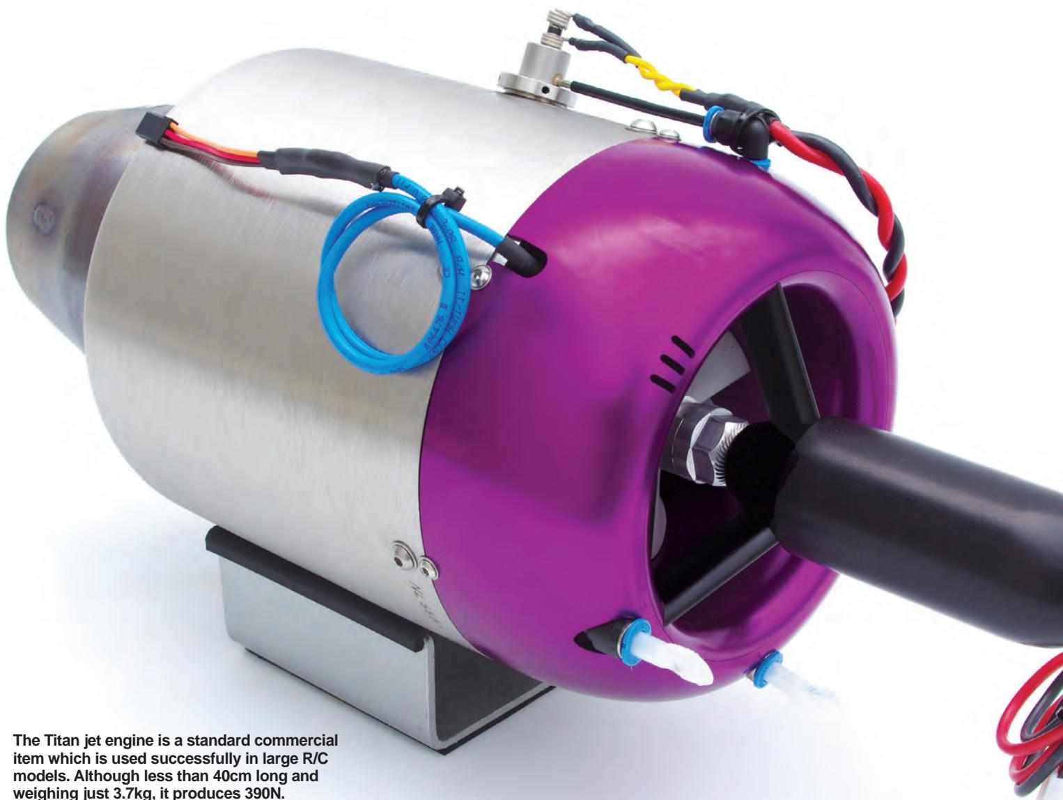
The Titan jet engine is a standard commercial item which is used successfully in large R/C models. Although less than 40cm long and weighing just 3.7kg, it produces 390N.
