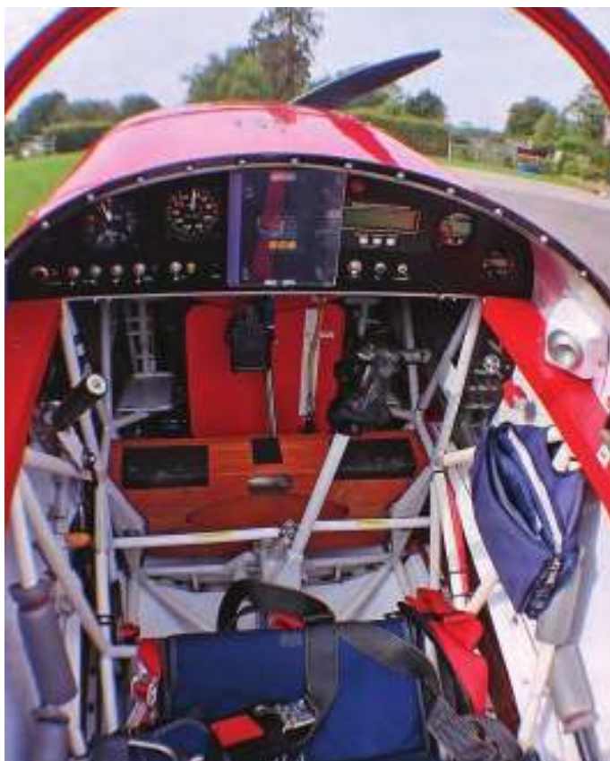
(Above) The panel of G-CVII features Dynon FlightDEK-D180 'glass', Trig Mode-S and a Becker 8.33 radio
