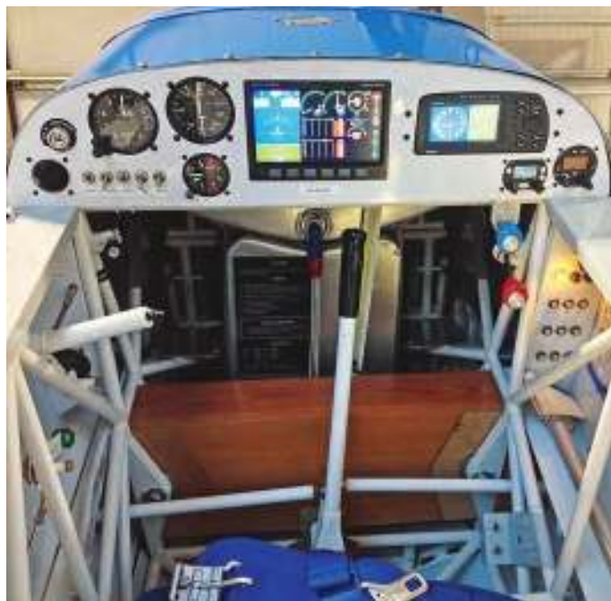
(Above) The panel of G-CVII features Dynon FlightDEK-D180 'glass', Trig Mode-S and a Becker 8.33 radio
