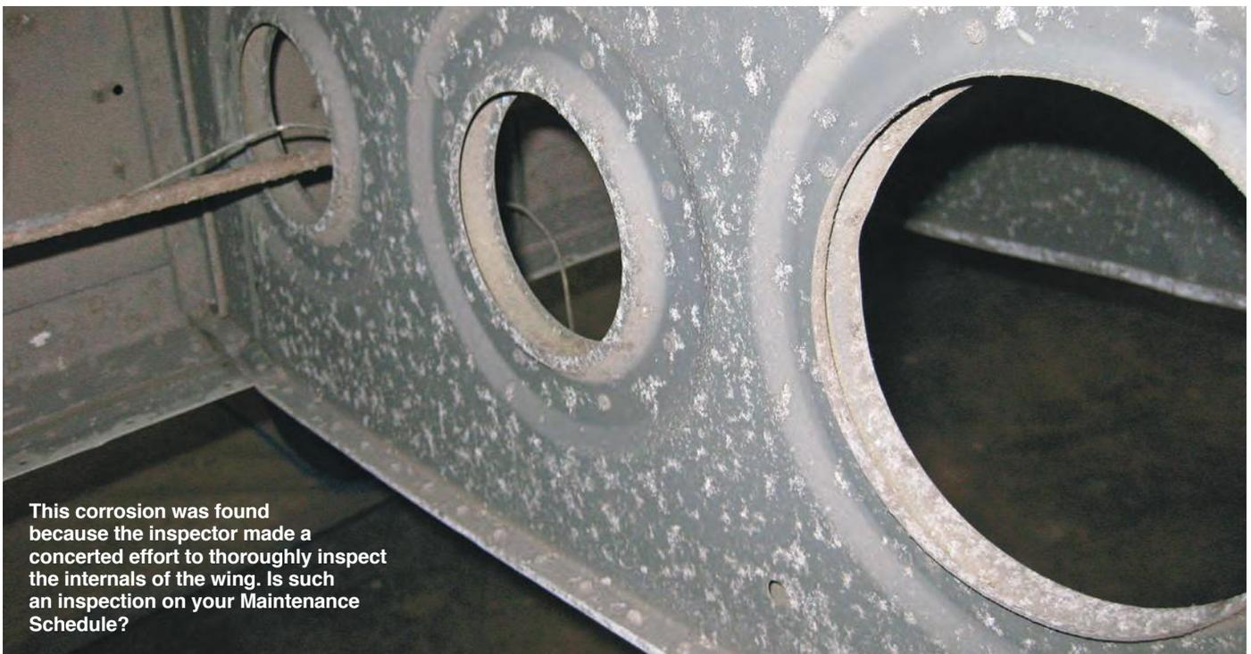
**This corrosion was found because the inspector made a concerted effort to thoroughly inspect the internals of the wing. Is such an inspection on your Maintenance Schedule?**
