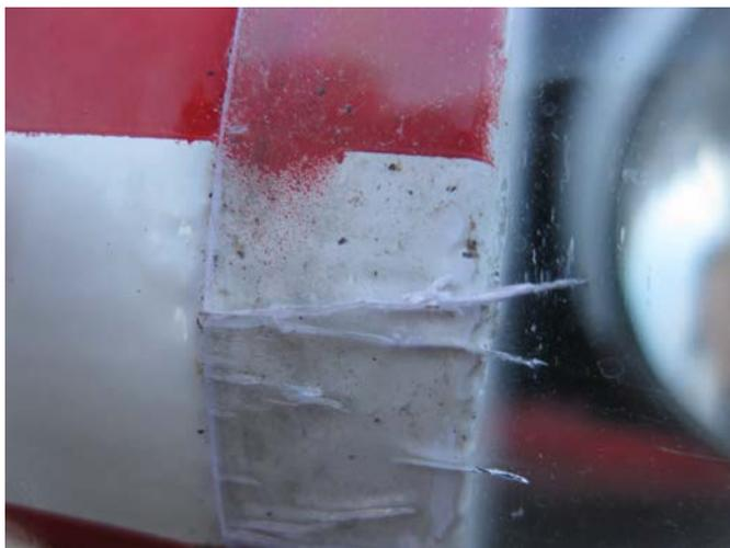
Fig 2. This picture shows an example of stress induced crazing which can lead to a local crack and subsequent failure of the part; this leading edge crazing has been caused because the part hasn't been heat formed. Jodel owners should be mindful that, should this part eventually fail, its failure might generate unforeseen flight safety problems for the pilot.
