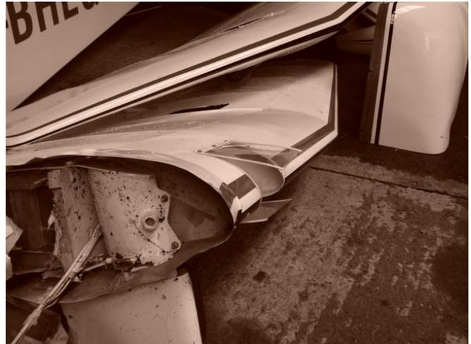
Fig. 1. The landing lamp cover fitted to this Jodel D150 Mascaret returned to its unformed shape, effectively a flat sheet, after failing in flight; this failure led to control difficulties for the pilot.
