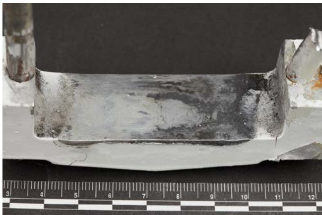
Fig. 2. Evidence of fretting due to loose U/C bolts
