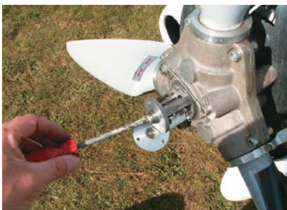
The location of the Leadscrew in the propeller hub
