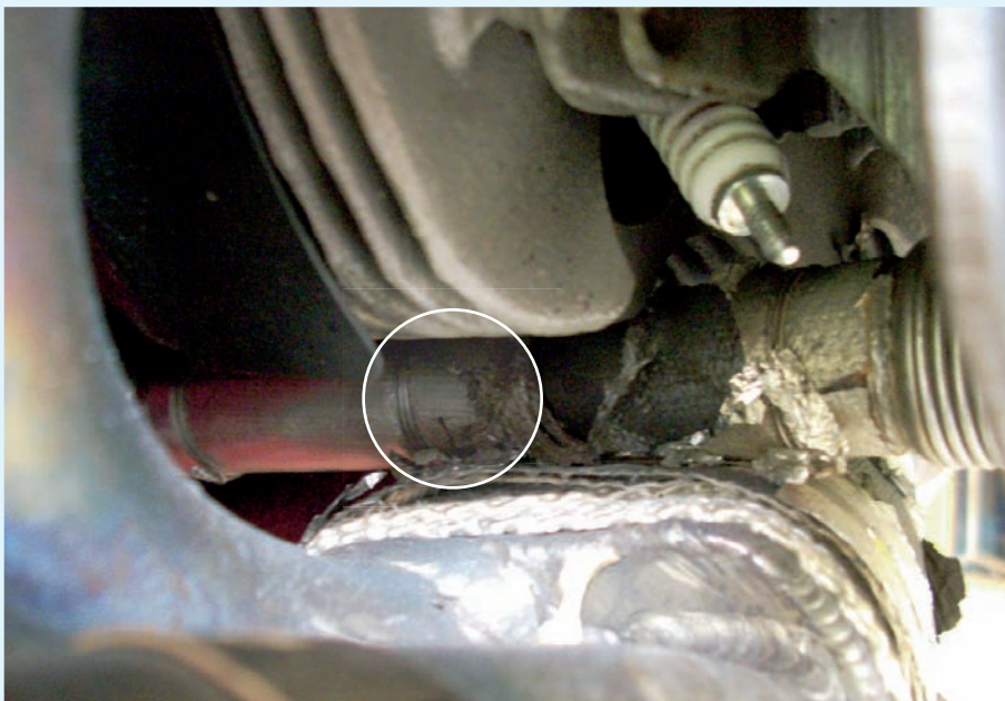
Gas flame can act like a blowtorch: Damage to push-rod tube shown above.
