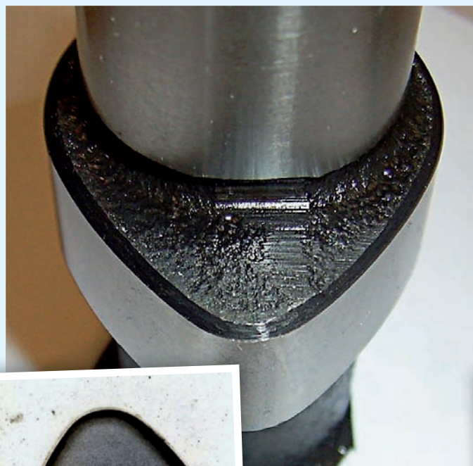
GOOD CAM: Note even chamfer around the edge of the cam lobe on this example of a new camshaft.
