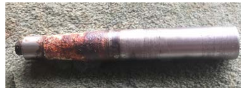
Fig 2. The picture above shows a badly corroded spindle removed from a modified (Dover Spindle Mod) undercarriage; the proposed AIL will require the spindle to be removed and inspected annually.
