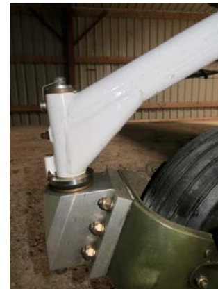
Fig 1. This picture shows a strengthened CZAW leg fitted with the Dover Spindle Mod; this undercarriage is fitted with a two 'leafed' fork, a three leafed alternative will be available shortly.
