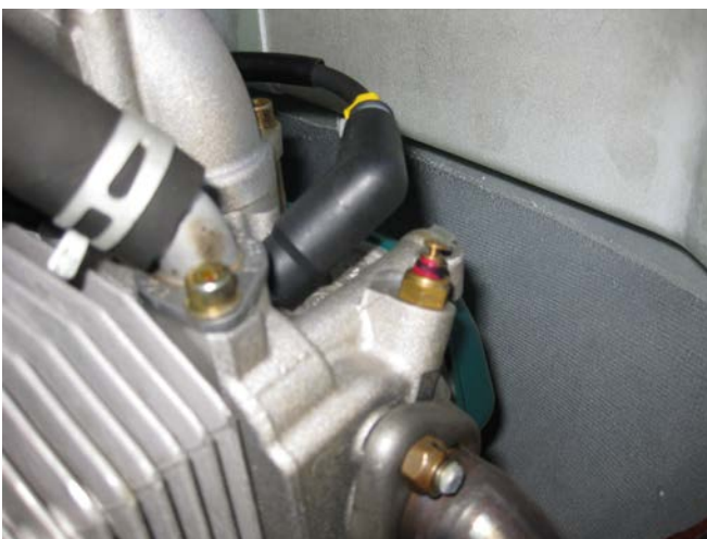
Fig. 2. Picture showing a post 2013 cylinder assembly designed to measure coolant temperature (CT); note that the sensor faces up.
