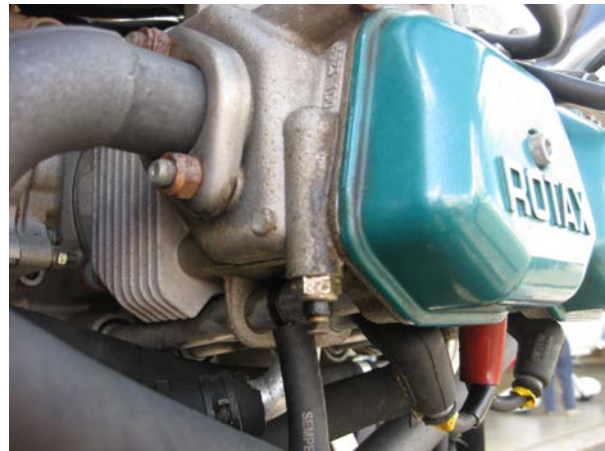
Fig. 1. Picture showing a cylinder manufactured before 2013 which measures Cylinder Head Temperature (CHT); note that the sender unit faces down.
