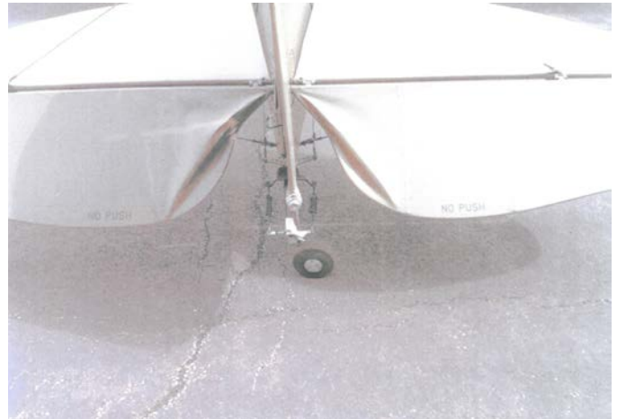
Fig. 1 A pilot of a J3 Piper Cub, whilst flying in the area of Leeds East (Church Fenton) airfield, started to feel a vibration through his rudder pedals, this was shortly followed by a bang and the aircraft pitched nose down. The throttle was closed and, with heavy stick forces, the aircraft was recovered back to level flight. The aircraft landed safely soon after; the picture above shows the damage caused to the elevators after this partial loss of control incident.
