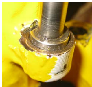
Fig. 2 (Left) shows that, under some circumstances, the head of the hinge pin can be smaller than the inside diameter of the hinge knuckle, this means that the hinge pin is only retained in place by the interference fit of the bearing (not visible). Fig.3 (Right) shows a simple 'fix' which will prevent the assembly failing should the bearing become loose; note the thin washer under the head and between the knuckle and the securing split pin.
