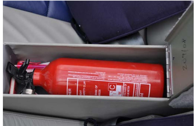
Fig. 1. It is essential that any article carried in the cockpit of an aircraft is properly restrained. A Fire extinguisher, if carried, must be affixed by an appropriate fixing to an appropriate structure.
