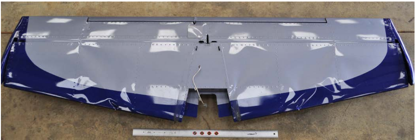
Fig 2. Shows the bottom surface of the SportCruiser's tailplane after suffering an in-flight structural failure.
