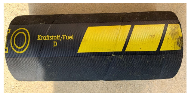
Fig. 2 This picture shows an example of a higher quality fuel hose which remains in perfect condition after many years' service. It can be seen that it is clearly marked as suitable for use with fuel. Should a pipe of this quality be fitted to an aircraft under inspection then, at the discretion of the LAA Inspector, the inspection frequency for this part may be reduced to every three years.
