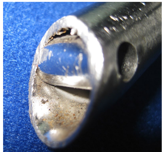
Fig 2. A 'close-in' picture showing the worrisome pitch control tube's end. As you can see, there's very little land between the through-bush and the end of the tube itself; there should be a minimum of 3 mm land here according to drawings of the part.
