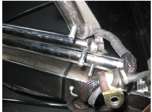
Fig. 1 This picture shows the base of the forward control stick with the starboard connection plate removed (for clarity). The stick itself pivots fore and aft, around the bottom bolt in the system and controls pitch; the bottom tube in the assembly has a bearing at each end which allows for side to side movement of the stick (roll).
