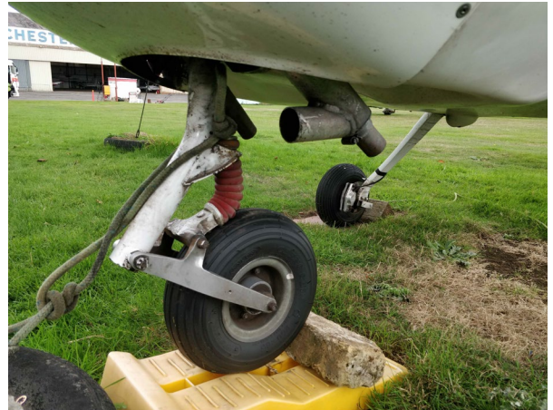
Fig. 1 The picture above shows the failed nose-undercarriage shock strut assembly; this strut has failed as a result of overload because of a heavy landing.
