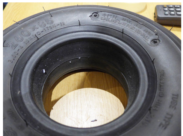
Fig. 2 This picture shows how the tyre looks when removed from the wheel assembly, note the very professional look to the inner infill core – and the fact that the tyre gives a maximum inflation pressure though, naturally, an inspector wouldn't find an inflation valve.
