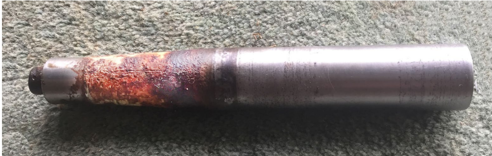
Fig 1. This picture shows the corrosion damage that has occurred unseen in a CZAW SportCruiser noseleg spindle after five years in service. Corrosion like this is extremely dangerous because surface corrosion pitting in high-strength steel is a common cause of cracking and component failure.
