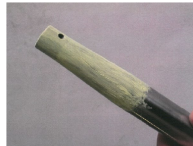
Fig 2. To act as a barrier between the mating surfaces a jointing compound is applied before assembly. When 'wet assembled', this has the added benefit of filling any voids which may allow water ingress into the assembly.
