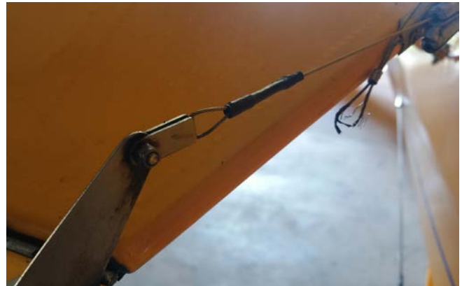
Fig. 1. This picture shows the detached bottom trim operating cable with the top cable still in place. Notice that the cable is forced around a sharp 90° angle: each operation requires the cable to go through an angular change causing fatigue in the individual strands.
