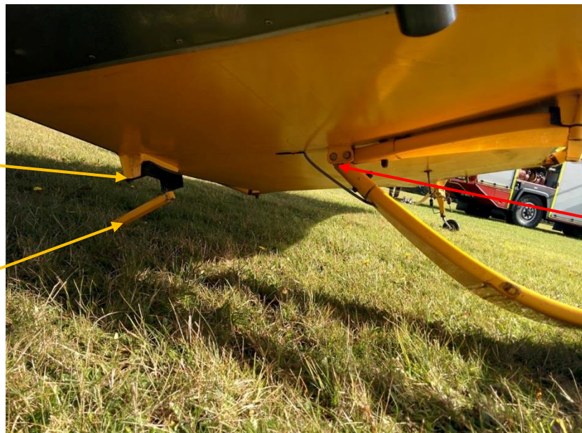
View of the undercarriage clamp bracket assembly (tail wheel aircraft)
