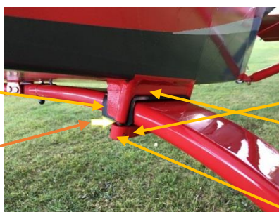
View of the undercarriage clamp bracket assembly (tail wheel aircraft)
