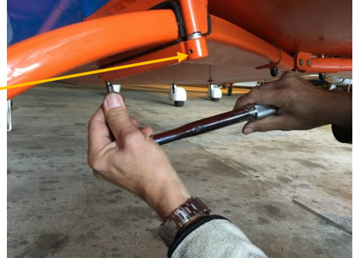
Clamp bracket locating hole
