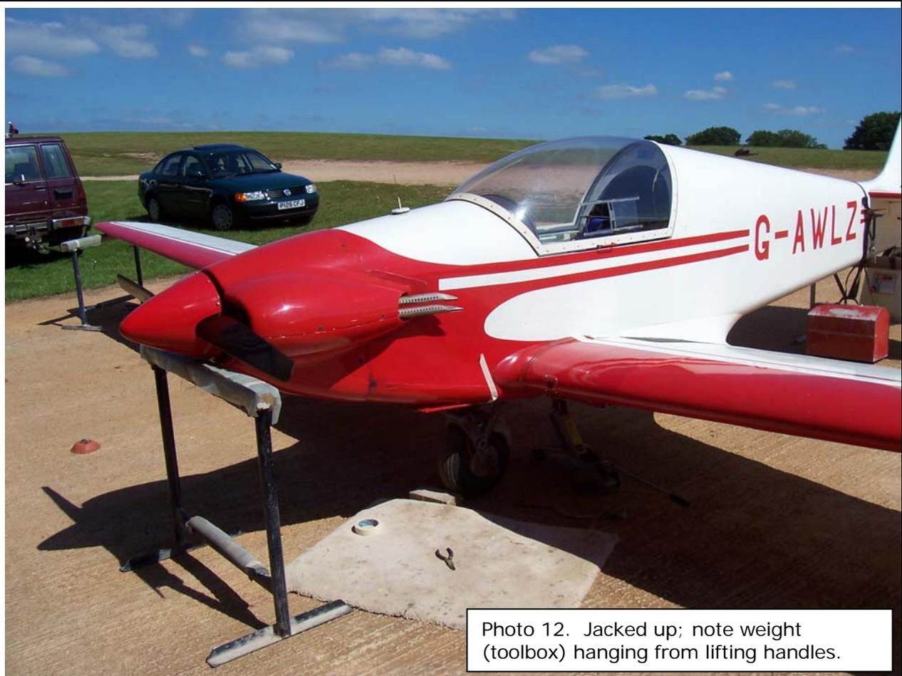
Photo 12. Jacked up; note weight (toolbox) hanging from lifting handles.
