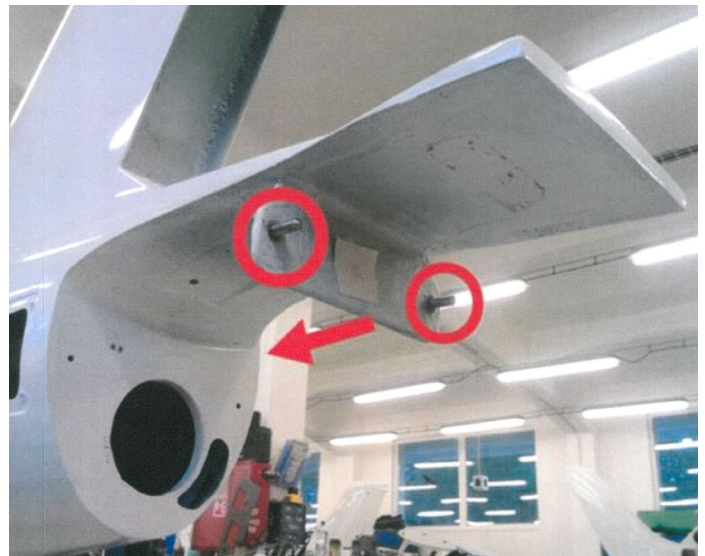
Fig. 1 This picture (above) shows the position of the two horizontal stabiliser's securing pins on the TL-Sting aircraft. Note that the stabiliser is finally secured using an attachment bolt at the forward end of the stabiliser. Inspectors should note that, because the bolt's head mates against the angled face of the stabiliser, a wedged-shaped washer is used – it is essential that this washer is fitted correctly.
