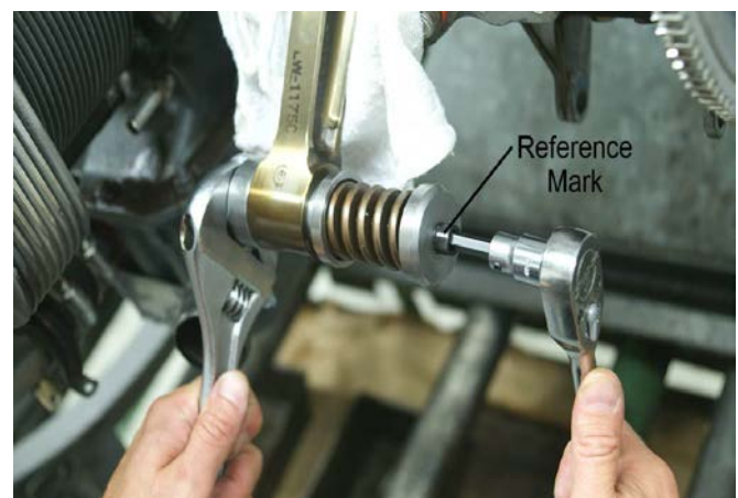
Fig. 2 The issue that's causing the trouble is that there appears to be a loose fit between the small end bearing and the connecting rod, though whether the error resides with one or both components is not known. This Lycoming tool tensions the bearing to check for a correct fit.
