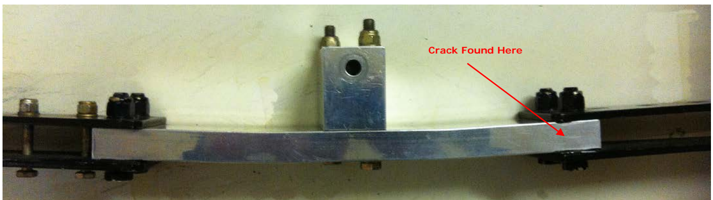
Fig. 2. Hub Bar Assembly minus Blades
