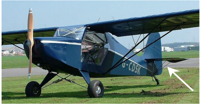
Figure 1: Escapade showing location of affected strut.
