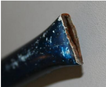
Figure 4: Fracture surface (strut removed from aircraft)
