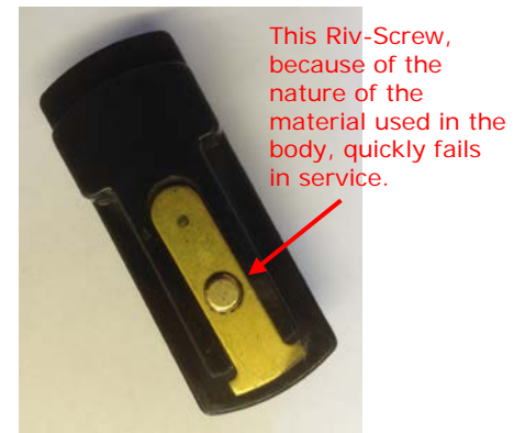
Fig. 2. This picture shows the design type that has been specifically withdrawn from service.
