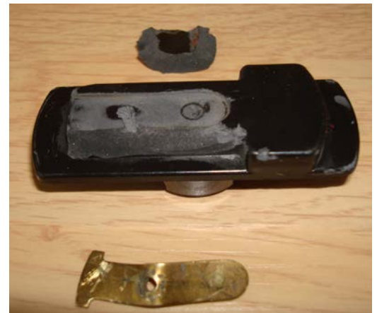
Fig. 1. An example of a 'typical' failure mode of a pattern Jabiru 2200 Rotor Arm.
