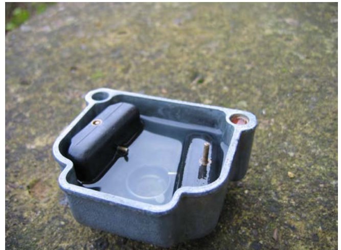
Fig. 1. This photo, taken in 2011, shows the difference in fuel absorption between the floats in a Bing carburettor (removed because the engine was running roughly). It's easy to check for problems here because the carburettor float bowl has been designed to be removed quickly (it's held on by a spring-clip).
