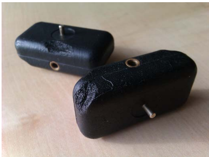
Fig. 2 The Tailored Maintenance Schedule (TMS) for your aircraft should include an inspection of the carburettor, this should be at least an 'Annual' check item. During this inspection it's certainly worth taking a close look at the floats: the first sign of problems of material failure in the example shown above was debris in the float bowl, although in this case the buoyancy of the floats wasn't noticeably affected.
