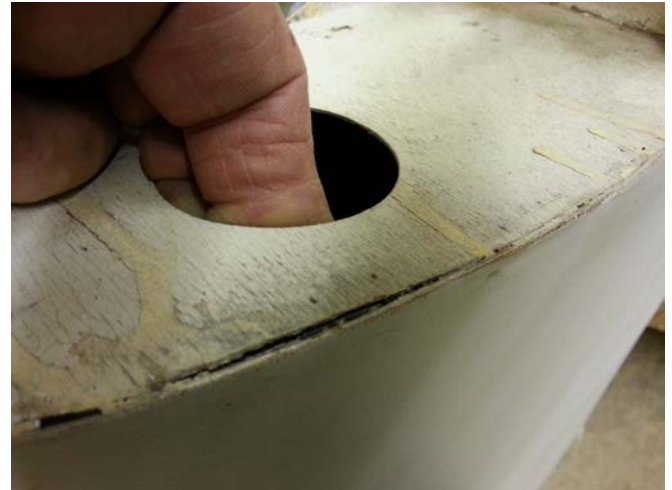
Fig. 1 This is a picture showing an inverted K8 fin; note that a very light pressure applied to the bottom rib reveals the failed glue joint. A complete failure of this joint could lead to the loss of the fin and compromise elevator control. (Picture courtesy of BGA)
