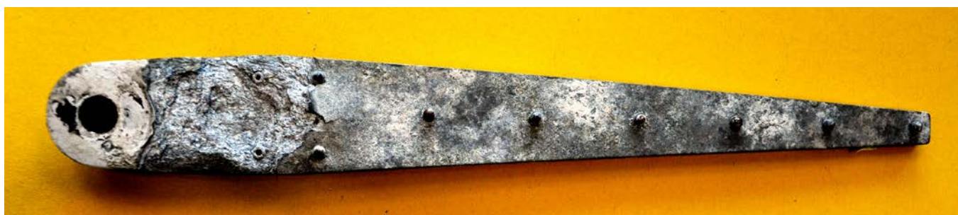
Fig. 2. In 2011, an MCR-01 forward wing attachment fitting fell off the wing whilst de-rigging the aircraft in preparation for re-painting; the corrosion present throughout the attachment surfaces and the failed attachment rivets are clear in the picture above. LAA Engineering produced an Airworthiness Information Leaflet (AIL) requiring immediate and then subsequent (3 yearly) de-rigs so that wing attachments could be checked: this AIL was mandated by a CAA MPD in April 2011.
