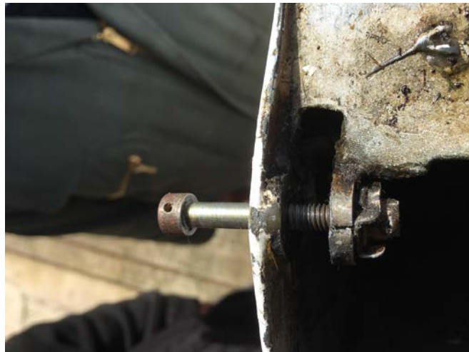
Fig. 1. This picture shows clearly that one lug in this tailplane attachment bracket has failed. The discovery of this failure came about by accident when an observant LAA Inspector noticed excessive play in the tailplane of the aircraft as it was being moved in its hangar.
