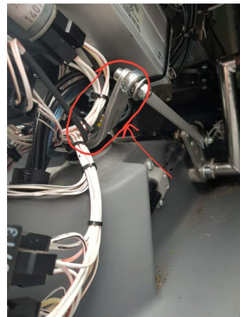
Fig 1. (Left) This picture shows the result of an overload to the top steering plate which has significantly bent; this was most probably caused because of an incorrect rudder application by a student being forcibly corrected by the instructor. Since this failure the steering brackets on aircraft equipped for training have been strengthened.
