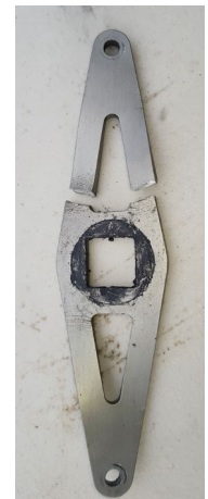
Fig 1. (Left) This picture shows the result of an overload to the top steering plate which has significantly bent; this was most probably caused because of an incorrect rudder application by a student being forcibly corrected by the instructor. Since this failure the steering brackets on aircraft equipped for training have been strengthened.
