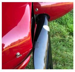
The owner of the Foxbat shown in the picture above noticed that the trailing edge of the propeller was very close indeed to the lower engine cowling, emphasising, perhaps, the great importance of a thorough pre-flight inspection.
