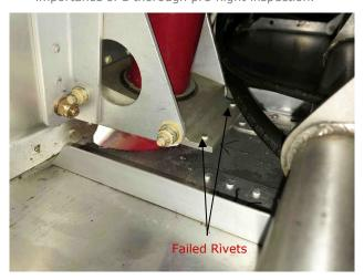
Further investigation revealed that the engine mount frame had moved because an essential structural element elsewhere had failed. Notice in the picture that both the rivets holding the nose undercarriage support block had broken. This block should have been held in place by four rivets and, because there were only two fitted, it failed under load far sooner than it was designed to.
