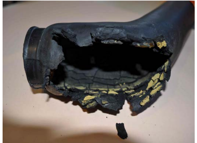
Fig 2. When the 'hidden' fuel filler pipe was removed from the aircraft it effectively disintegrated; it should be noted that the pipe looked from the outside to be in good condition (except, in this example, it was leaking fuel)
