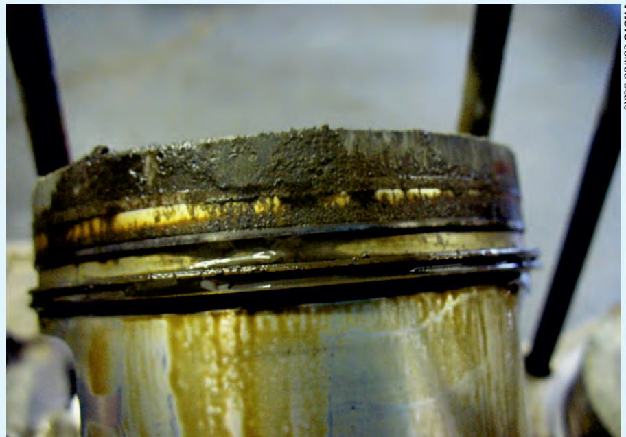
It can be seen that this piston's operation has been severely compromised by the lead compounds formed in this engine. The top piston ring is completely stuck in its groove.
