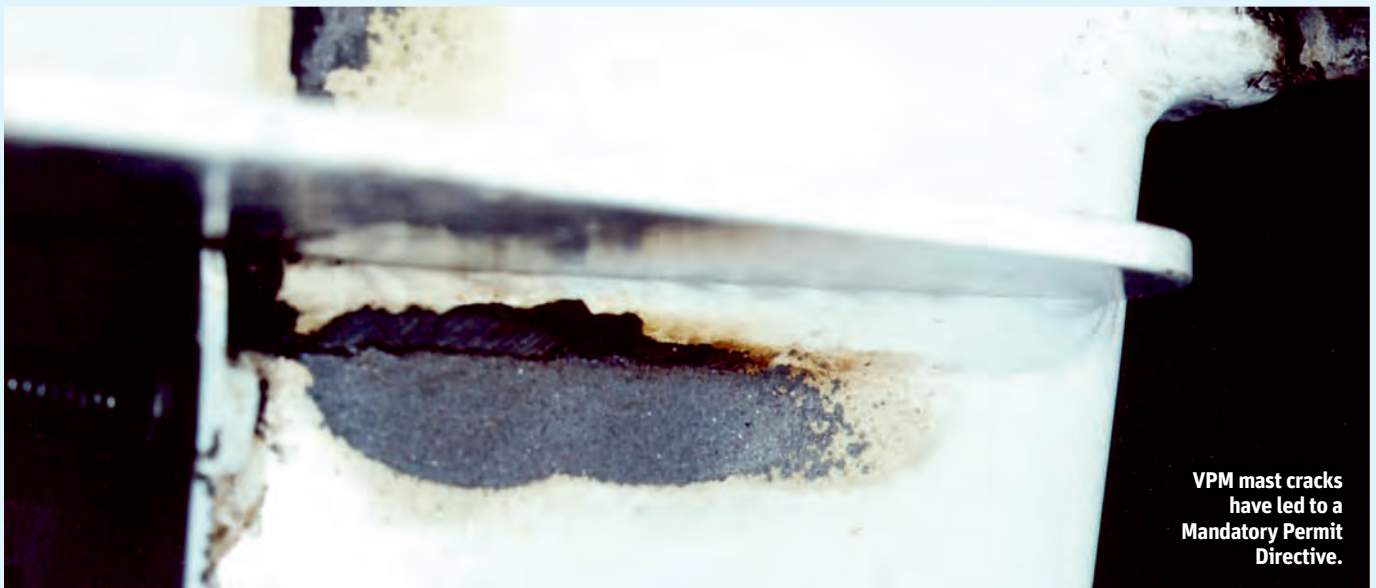
Some of the mast cracks are incredibly difficult to spot.
