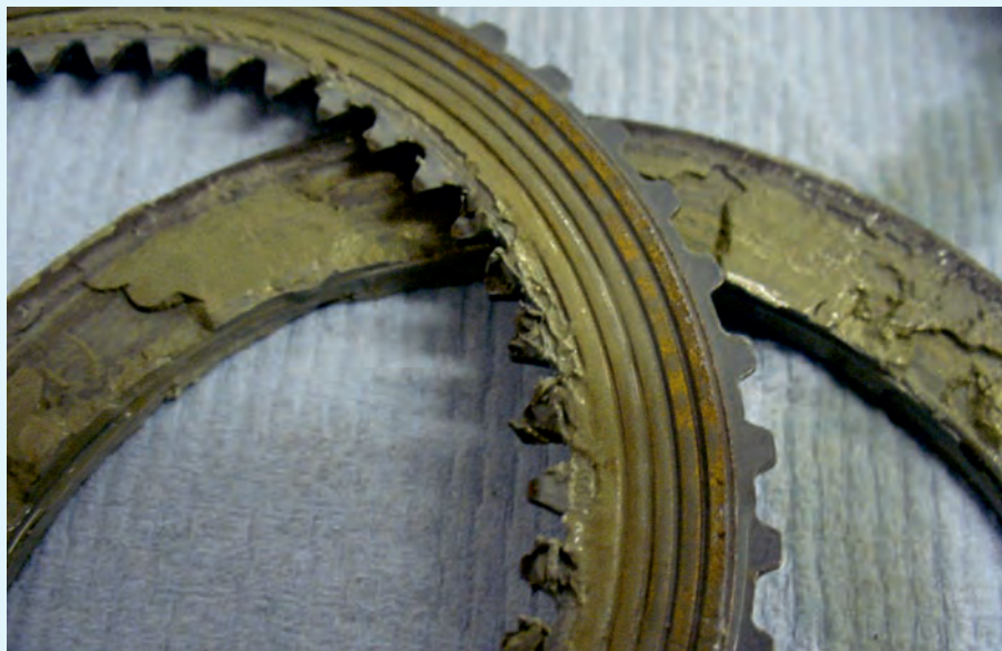
The clutch plates on this Rotax Overload Clutch – one of three 'clutches' on the engine – are completely full of lead based deposit. If this device was needed it probably wouldn't work.
