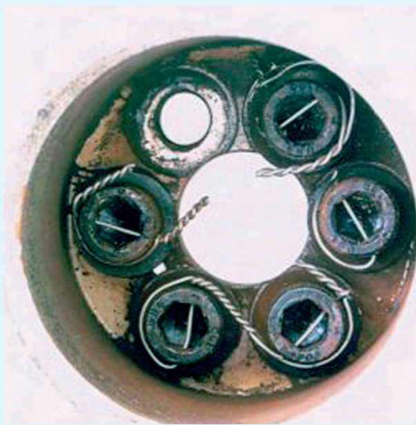
Impossible to see with the propeller fitted, but the wire locking has broken allowing progressive slackening of the bolts, leading to failure.
