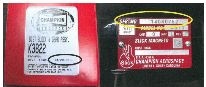
Fig 2. Distributor gears manufactured between 2008 and 2016 may contain suspect finger electrodes. The serial number, on the magneto's data plate, also contains the date of manufacture.
