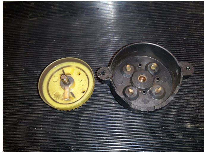
Fig 1. The 'finger' electrode directs the high-tension electrical charge to the correct plug at the correct time. Looseness in the electrode will affect the quality of the spark and may cause rough running. As the gap between the finger electrode and the contact in the distribution cap naturally increases with age, increased sparking will decrease the efficiency of the ignition system and may lead to a failure of one or more cylinders.
