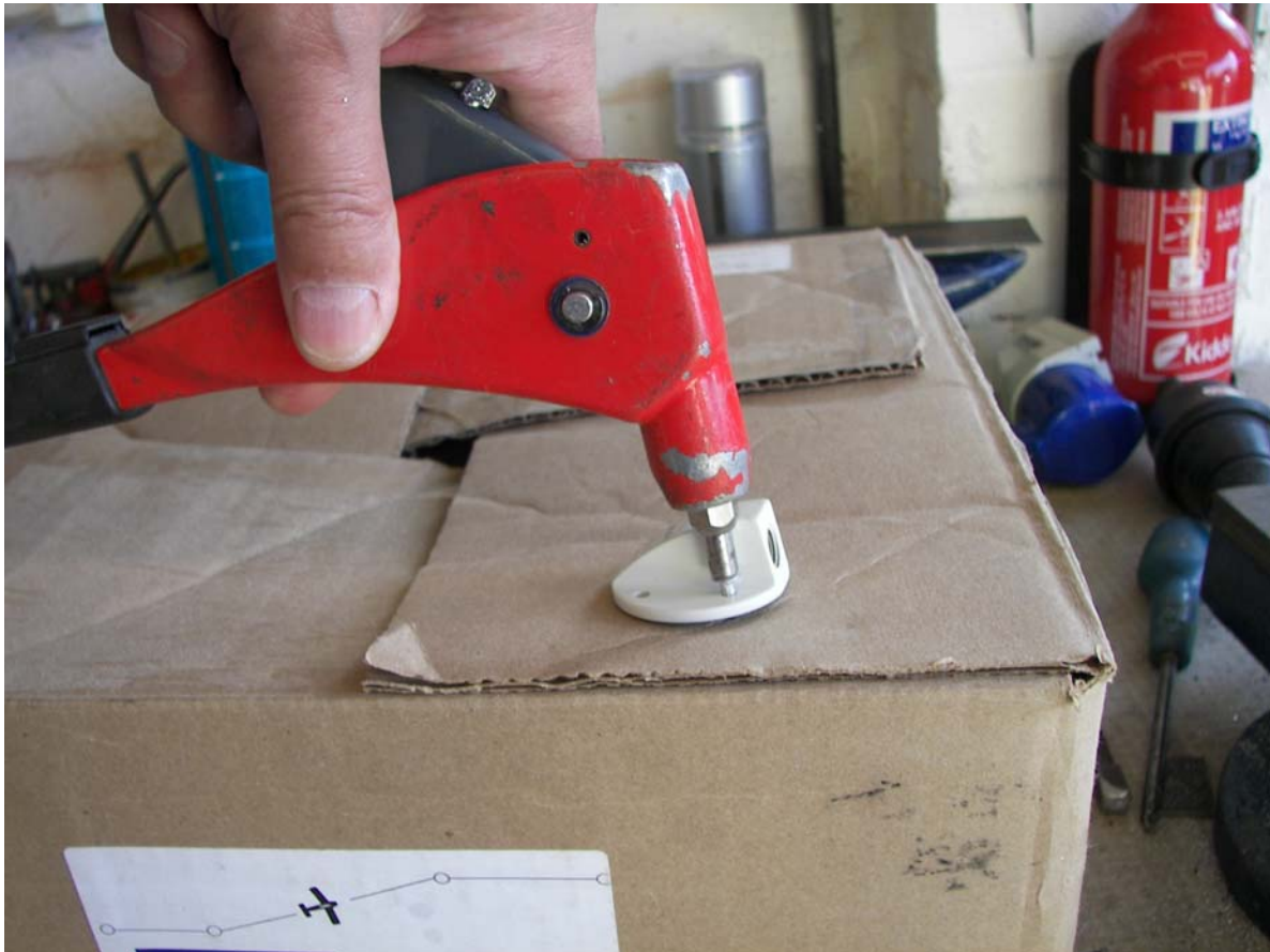
Note 10mm long adaptor to avoid clash between rivet gun and drain valve fitting.
