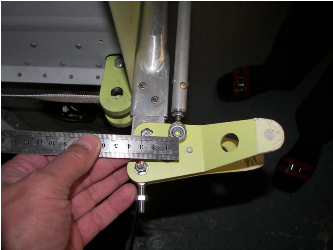
Fig 9. Elevator idler showing where servo push-rod attachment hole needs to be.
