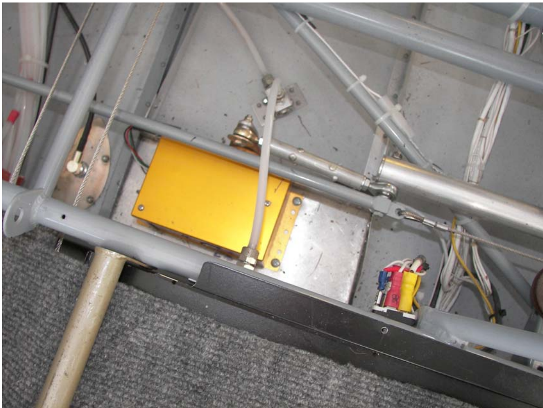
Fig 1. View looking down on roll servo.
