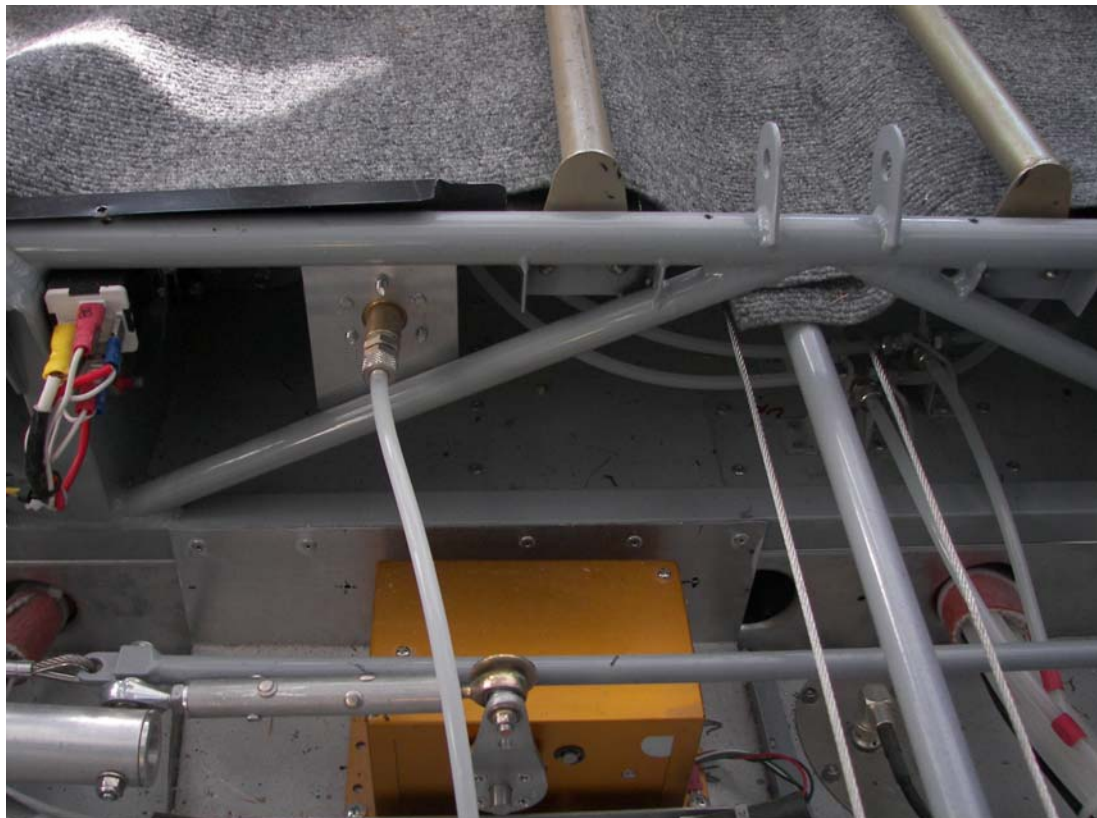
Fig 3. Roll servo viewed from behind.
