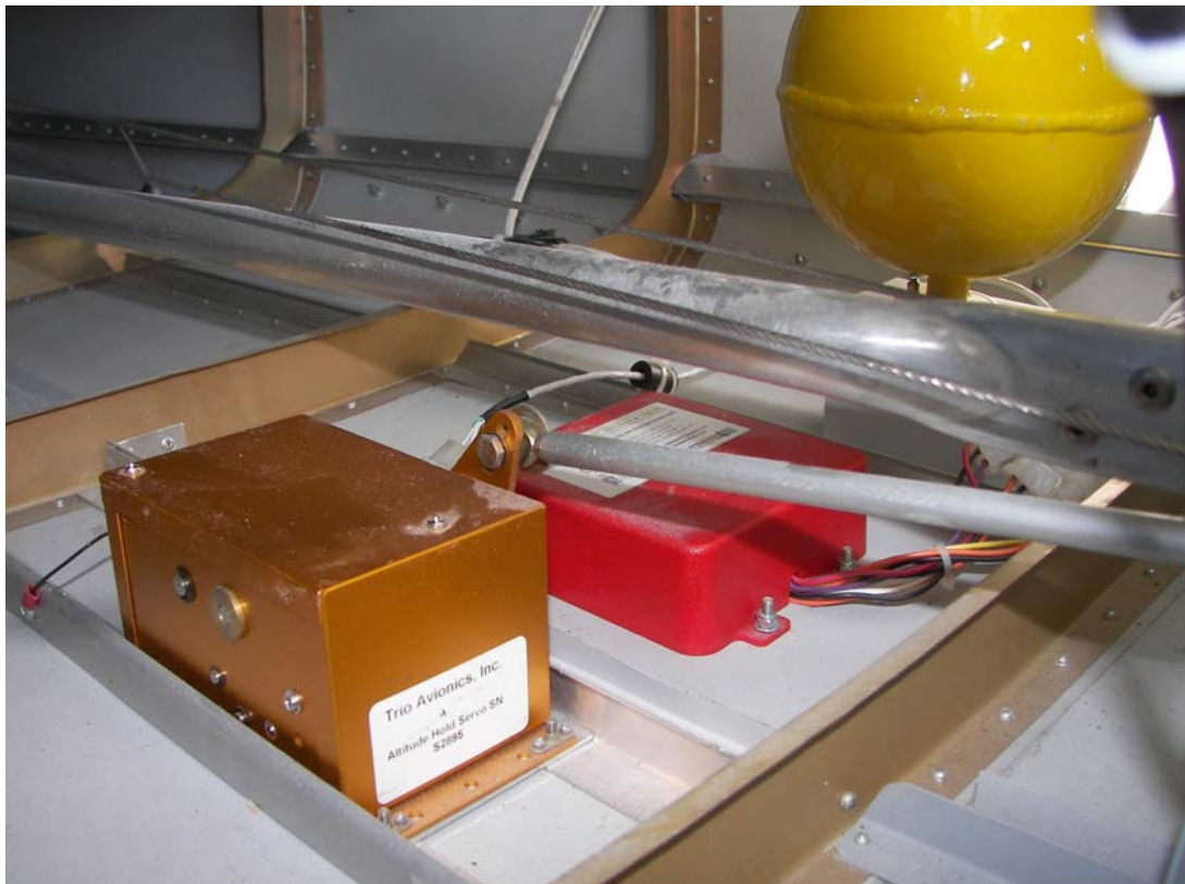
Fig 8 Pitch servo on mounting rails.
