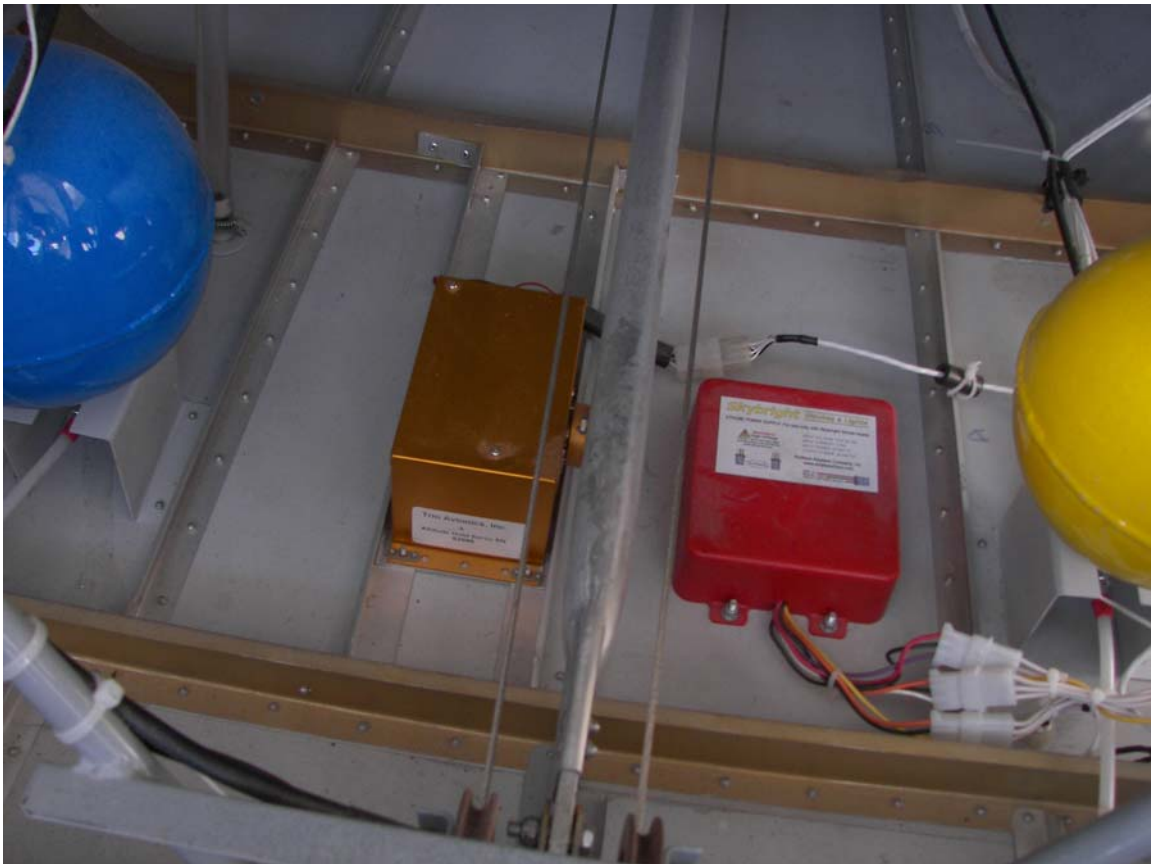
Fig 6. Pitch servo looking aft.
