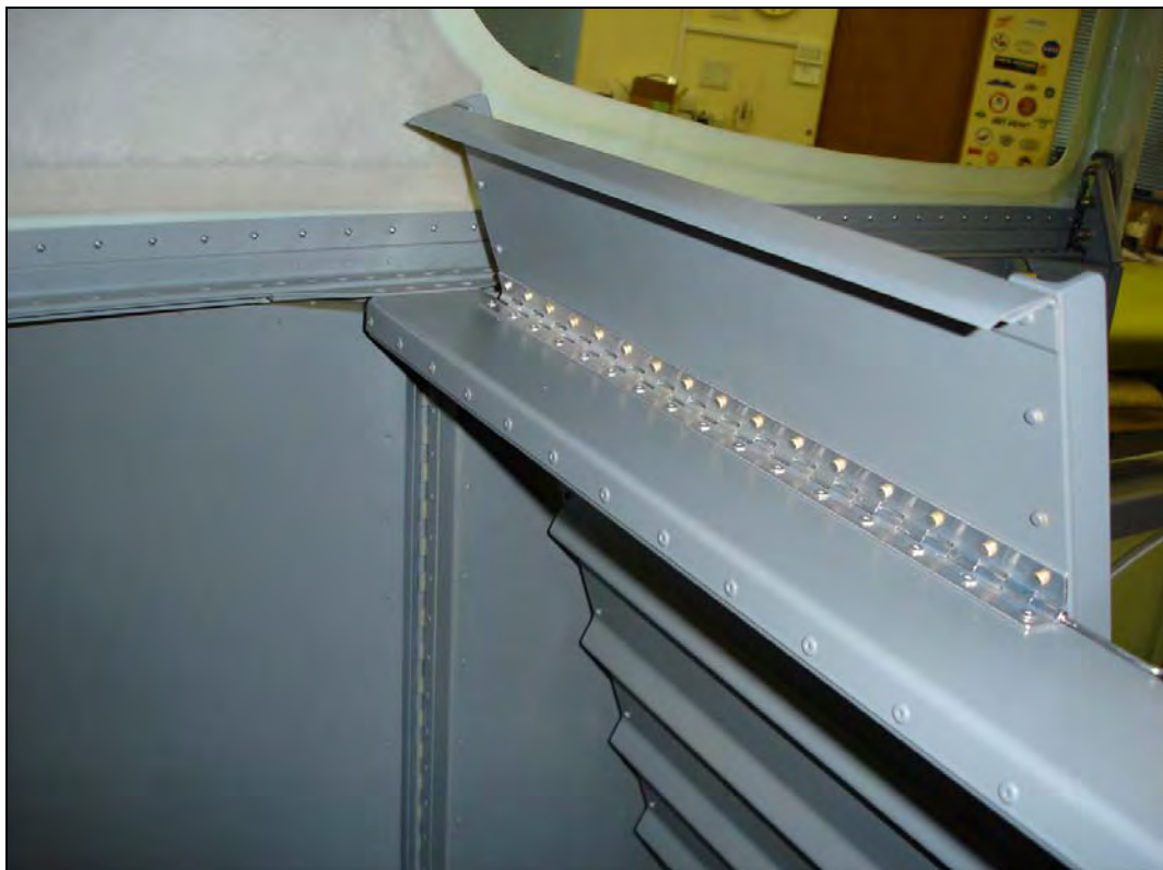
Picture 2 Port side, rear seat back with hinge riveted in position, view looking forward
