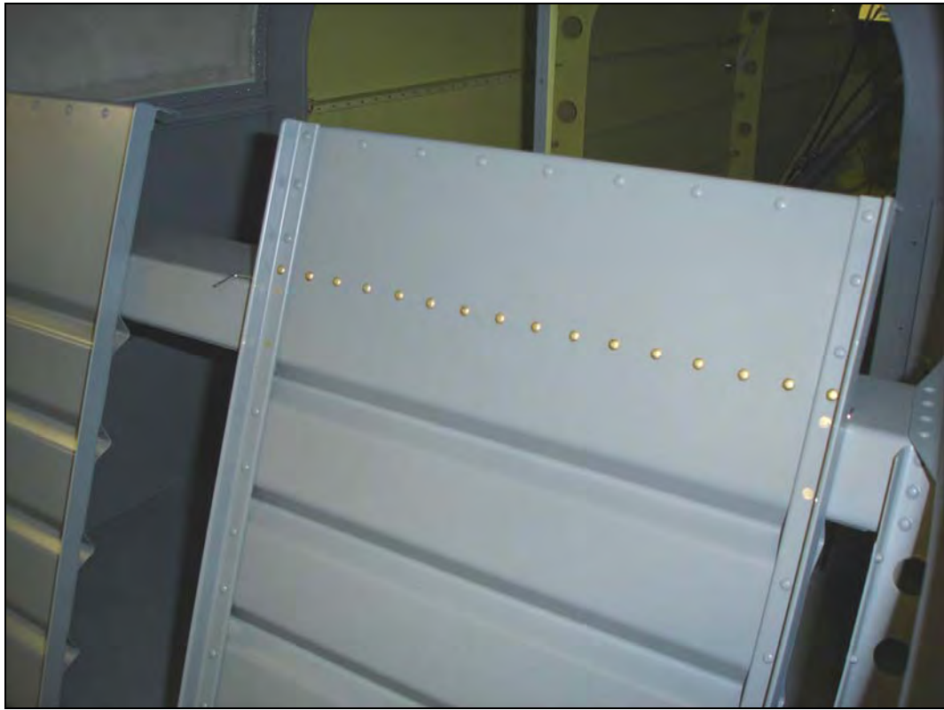
Picture 1 Port side, rear seat back with hinge riveted in position, view looking aft
