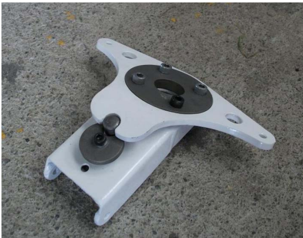
Tailwheel steering pin engaged.
