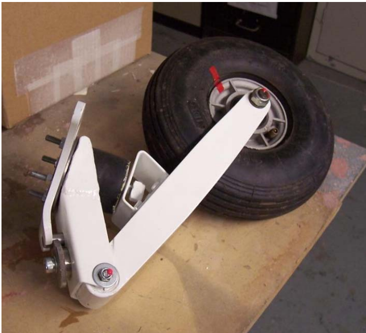
RF-5 Tailwheel assembly with castoring facility installed.
