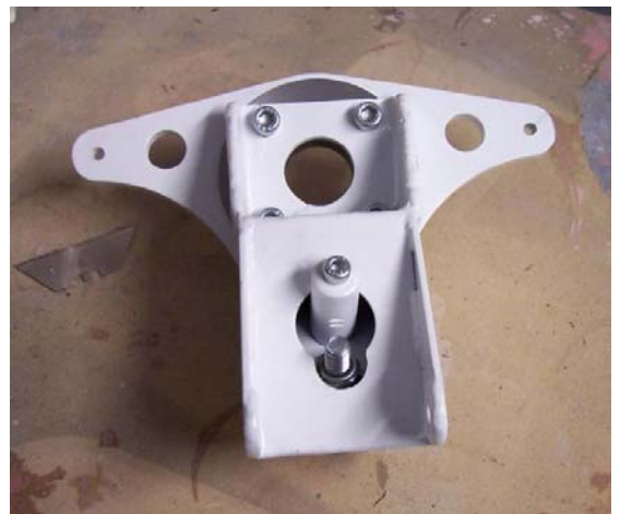
Underside of tailwheel support arm
