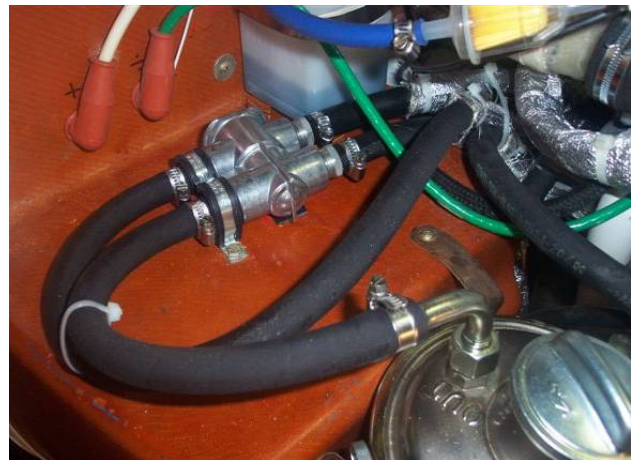
Figure 6 Example of valve installation in a Europa aircraft.
