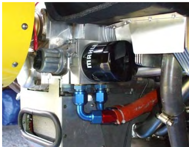
Typical neat installation with firewall mounted oil cooler
