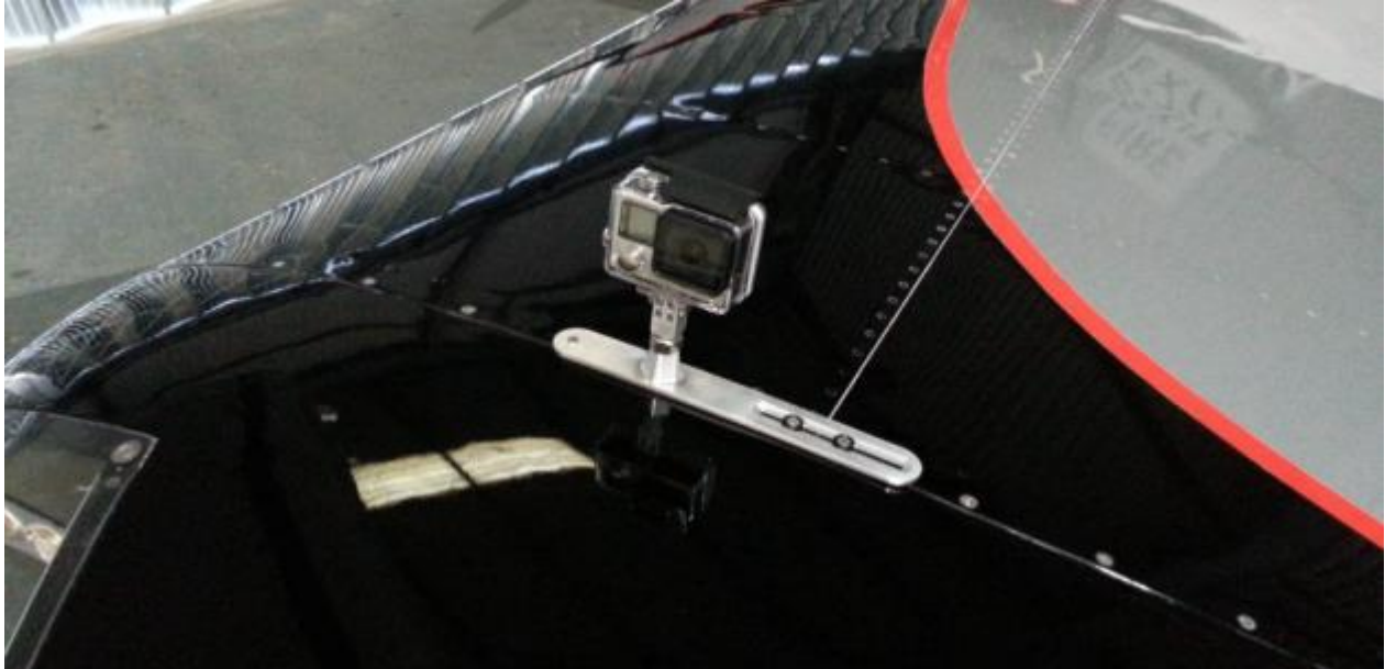
SM14083-02 Photograph of Installation – Wing Tip Mount Close Up
