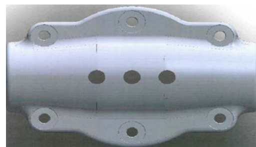
Fig 3. This picture shows the front half of a later model 2A0 propeller hub (Revision 'E' and later). This model hub (and the three blade equivalent) are not affected by SB2016-06B
