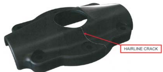
Fig 2. This picture shows the front half of the earlier model 2A0 propeller hub (Revision 'D' and earlier). Cracks appear to be originating from the pitch setting marks impressed into the hub; it is essential to remove the hub to inspect as hairline cracks may be difficult to spot.
